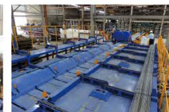
Rebar Feeder with Separators
